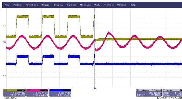
Fig. 10 Effect of ESD at ZCD output for 15kV
