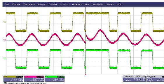
Fig. 13 Effect of ESD at oscillator output for 8kV.
