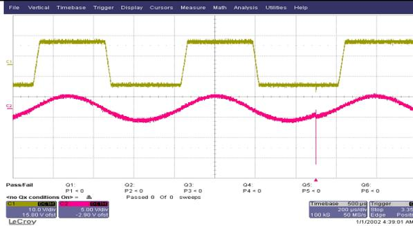
Fig. 5 Effect of ESD at 15kV and at a distance of 0.9m
