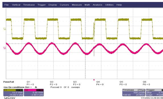
Fig. 7 Effect of ESD at 8kV and at a distance of 0.5m
