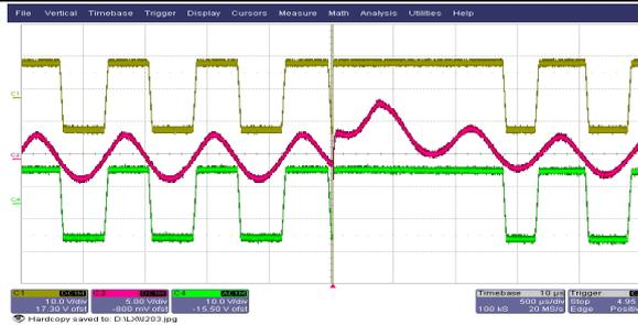
Fig. 14 Effect of ESD at oscillator output for 15kV
