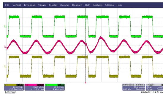
Fig. 11 Effect of ESD at oscillator output for 2kV
