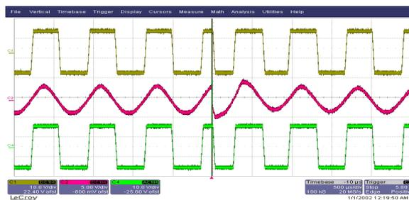
Fig. 9 Effect of ESD at ZCD output for 4kV
