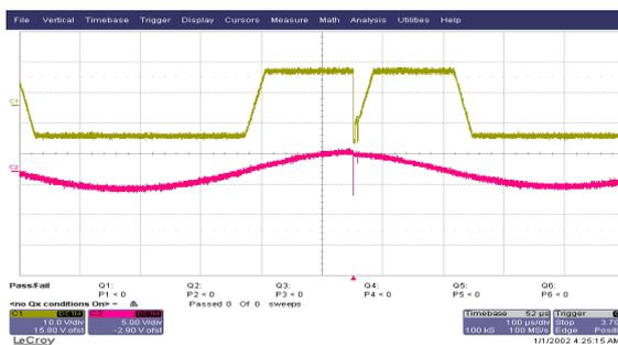
Fig. 4 Effect of ESD at 8kV and at a distance of 0.9m
