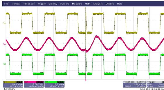
Fig. 8 Effect of ESD at ZCD output for 2kV
