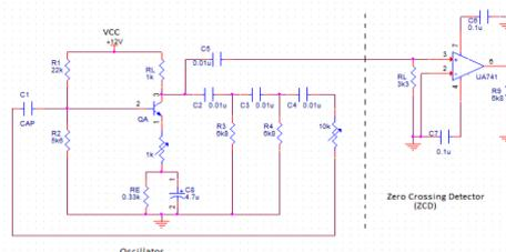
Fig. 1 Circuit diagram of RC phase-shift oscillator followed by zero crossing detector.
