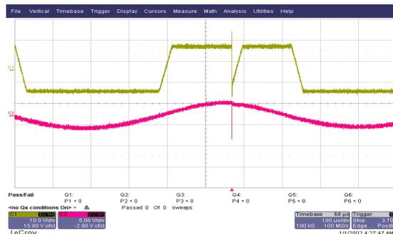
Fig. 6 Effect of ESD at 8kV and at a distance of 0.7m
