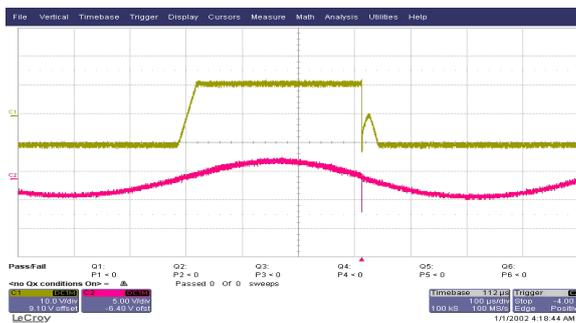
Fig. 3 Effect of ESD at 4kV and at a distance of 0.9m
