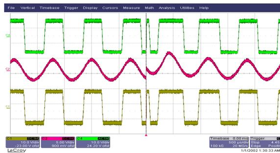
Fig. 12 Effect of ESD at oscillator output for 4kV.
