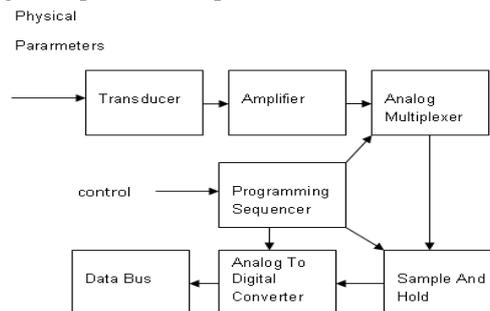
Figure 1: Data Acquisition System
