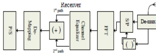
Fig 3(b) Receiver of PRCC technique
