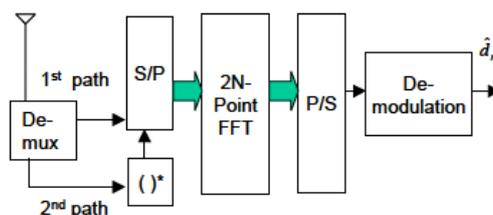
Fig.2(b) Receiver of CC scheme
