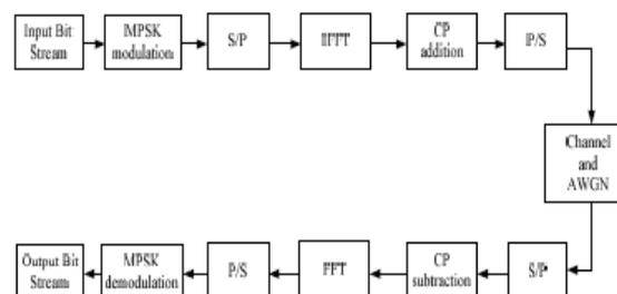
Figure 1: Block diagram of a baseband OFDM System
