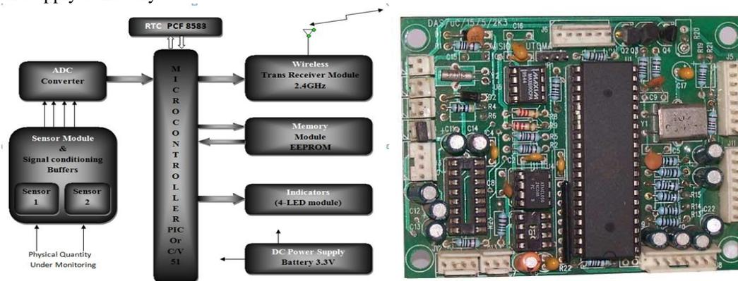
Fig. 2. Schematic Block Diagram for Remote Monitoring Smart Node & Slave Node HW (PIC 16F877)
