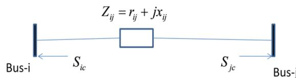
**Fig. 2. Injection model of TCSC**
