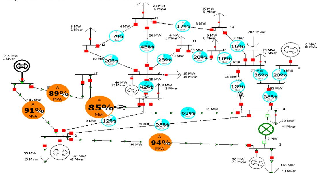
**Fig .10. Modified IEEE 14 bus system with TCPAR is placed in line 1-5**
