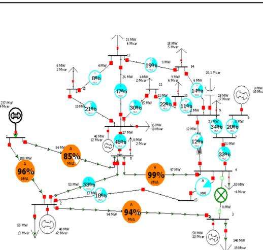
**Fig .12. Modified IEEE 14 bus system with TCPAR is placed in line 2-4**
