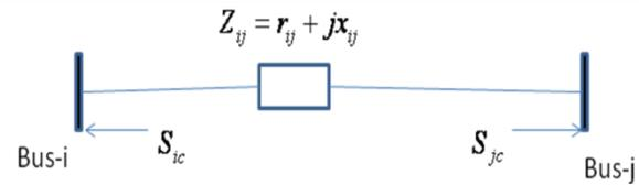
Fig.4. Injection model of a TCPAR
