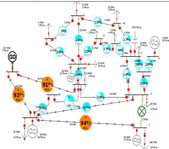
**Fig.11. Modified IEEE 14 bus system with TCPAR placed in line 2-5**
