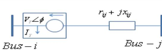
Fig.3. Equivalent circuit of TCPAR
