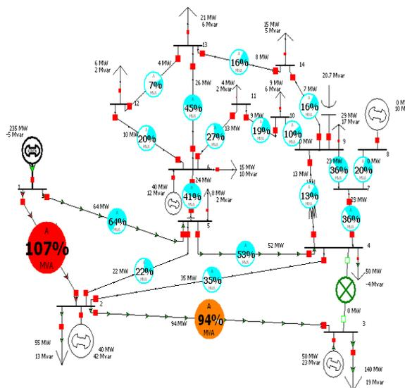
**Fig. 6. Modified IEEE 14 bus in which line 1-2 is overloaded when 3-4 line is outaged**
