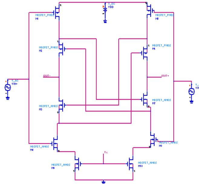
Figure 1: Feed forward Regulated Cascode OTA
