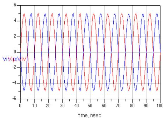
Figure 2. Differential Input Voltage in time domain
