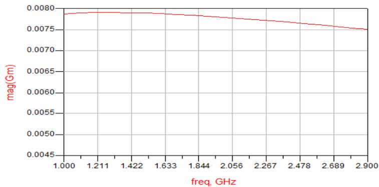
Figure 4. Simulated OTA's Transconductance
