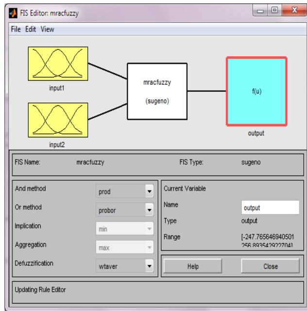
Fig 3.4 : Editor view of fuzzy controller in MATLAB/Simulink
