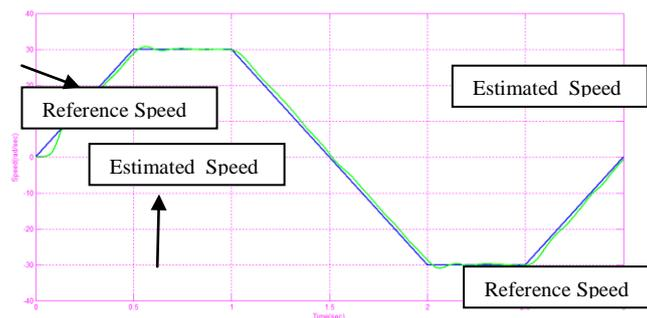
Fig 4.3: simulation results of reference and estimated speed
