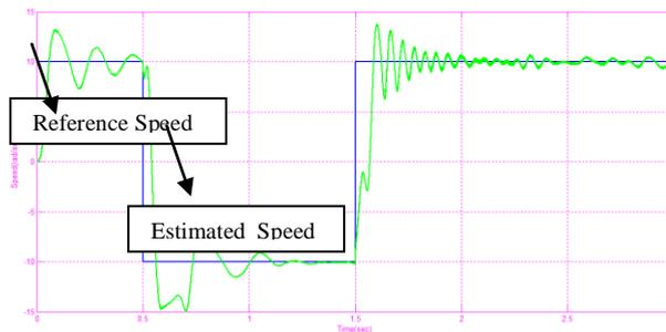
Fig 4.6: simulation results of reference and estimated speed
