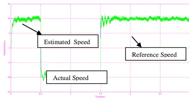
Fig 4.4: simulation results of reference and estimated speed
