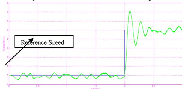
Fig 4.9: simulation results of reference and estimated speed
