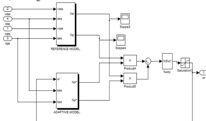
Fig 3.3 : Simulation model of MRAS with Fuzzy logic controller
