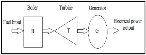
Fig.1 Simple model of thermal generation system
