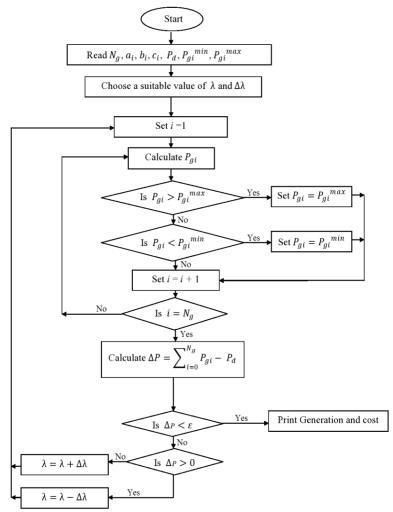
Fig. 2 Flow chart of lambda iteration method for ELD
