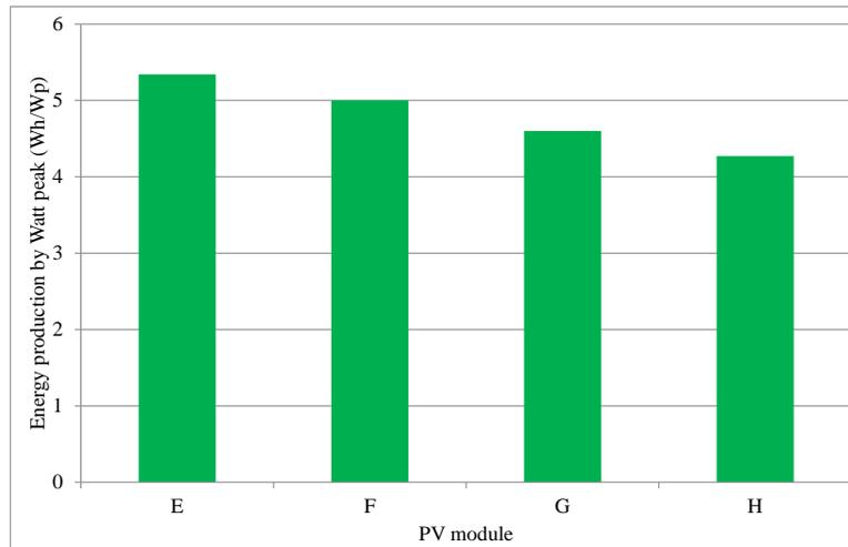
**Fig.17:**Energy production by watt-peak of the autonomous PV system of 24 V according to PV modules E, F, G and H
