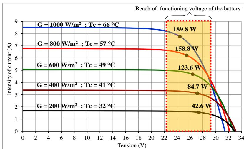
**Fig.13:**Position of the optimal functioning points of PV module (E) in relation to the beach of functioning tension of a battery of 24 V
