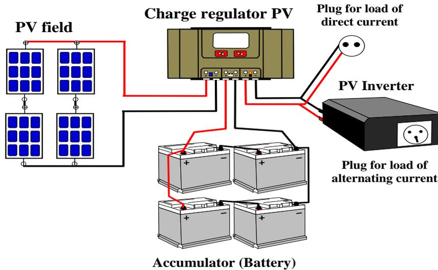
**Fig.1:** Representation of an autonomous PV system
