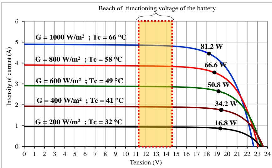
Fig.10: Position of theoptimal functioning points of PV module (C) in relation to the beach of functioning tension of a battery of 12 V
