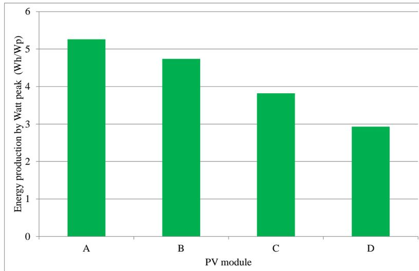
**Fig.12:**Energy production by watt- peak of the autonomous PV system of 12 V according toPV modules A, B, C and D
