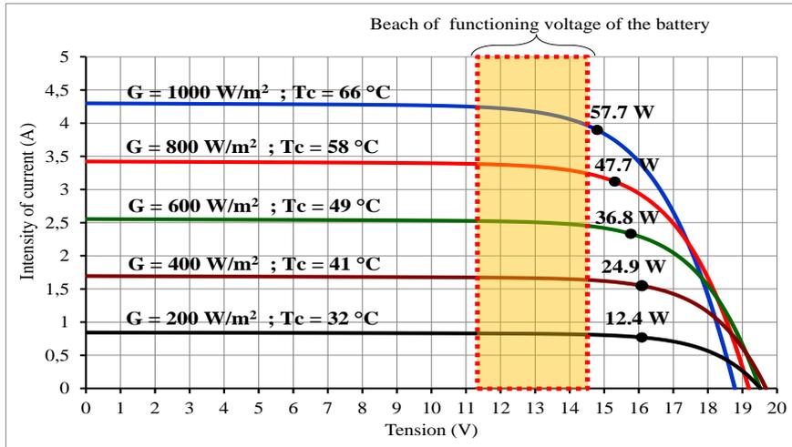
Fig.9: Position of theoptimal functioning points of PV module (B) in relation to the beach of functioning tension of a battery of 12 V
