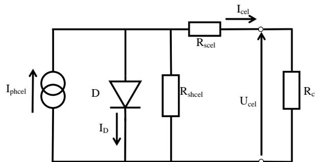
**Fig. 2:**Equivalent circuit of a photovoltaic cell
