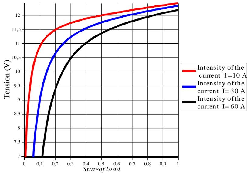
Fig.6:Curves of discharge of the lead-acid battery to different regimes
