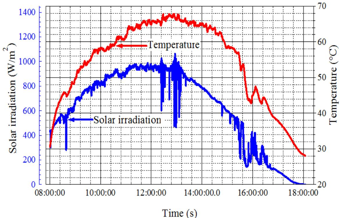
**Fig.5** Evolution of the solar irradiation and of the temperature of a PV module during one day
