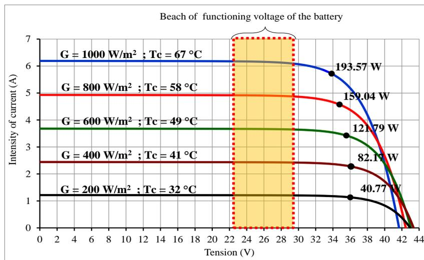
Fig.16: Position of the optimal functioning points of PV module (H) in relation to the beach offunctioning tension of a battery of 24 V
