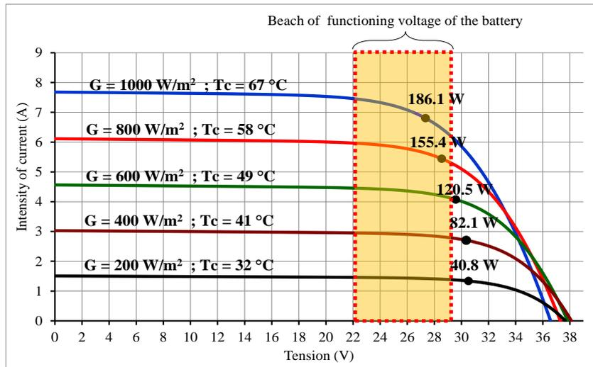
Fig.14: Position of the optimal functioning points of PV module (F) in relation to the beach offunctioning tension of a battery of 24 V
