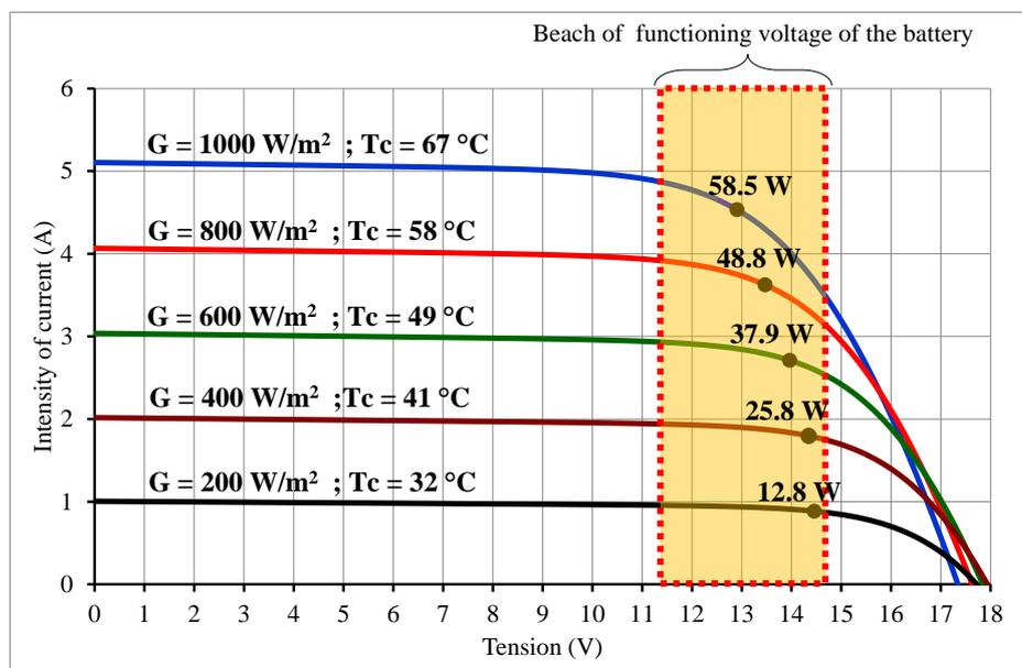
**Fig.8: Position of the optimal functioning points of PV module (A) in relation to the beach of functioning tension of a battery of 12 V**
