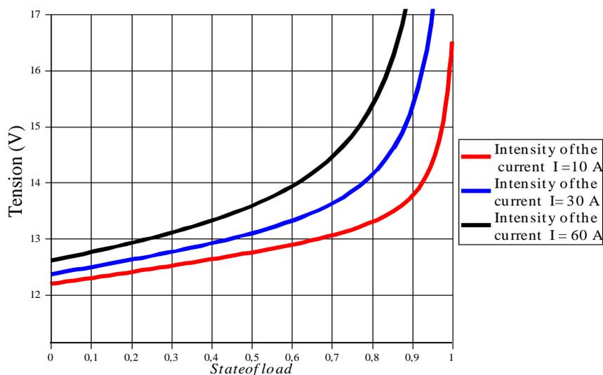
Fig.7:Curves of charge of the lead-acid battery to different regimes
