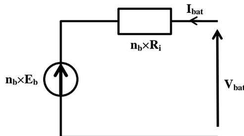
**Fig.3**Equivalent electric circuit of nb elements accumulator in series
