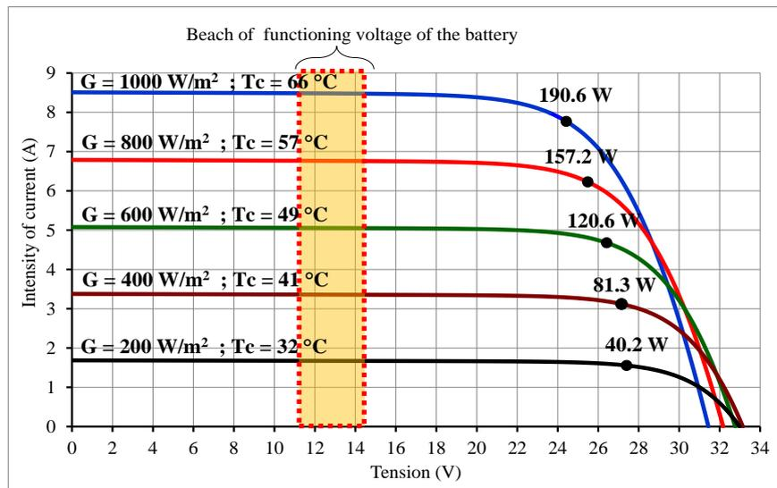
Fig.11: Position of theoptimal functioning points of PV module (D) in relation to the beach offunctioning tension of a battery of 12 V
