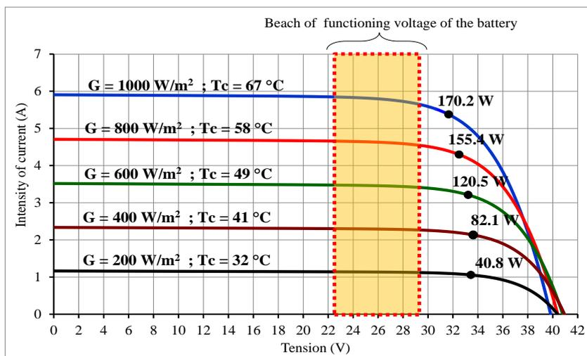
Fig.15: Position of the optimal functioning points of PV module (G) in relation to the beach offunctioning tension of a battery of 24 V
