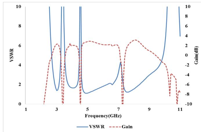
Fig. 8: VSWR and gain total vs. frequency plots of the geometry shown in Figure 7.
