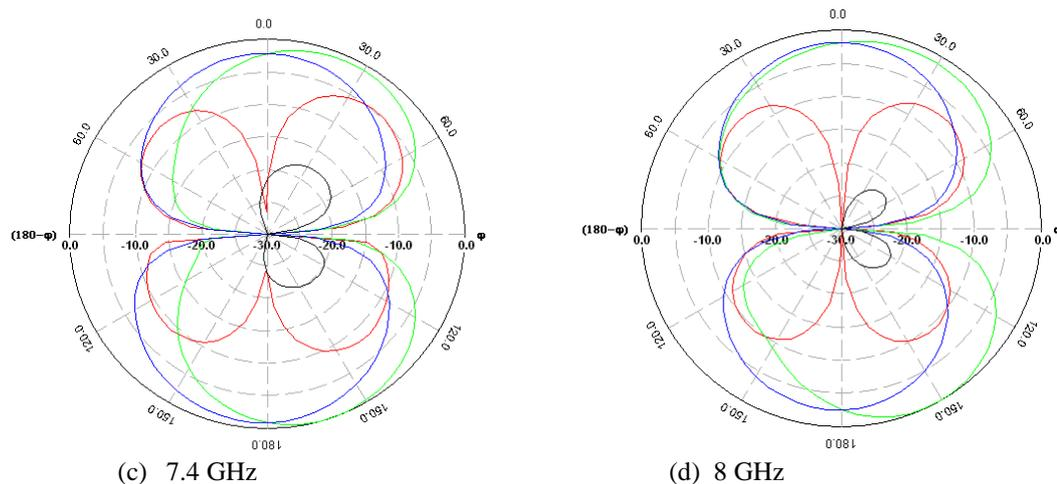
**Fig. 14:** E and H plane radiation patterns at different frequencies in operating bands. Note: Blue curve: H-Co. Poln.; Gree curve:E-Co. Poln.; Red curve: E-Cross Poln.: Black curve: H-Cross Poln.
