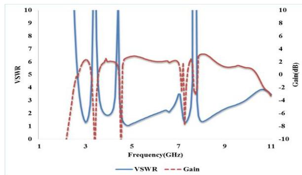
**Fig. 10:** VSWR and gain total vs. frequency plots of the optimised geometry shown in Figure 9.
