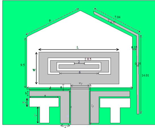
**Fig. 9:** Four bands notch optimised antenna
