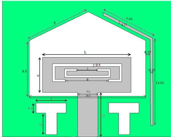
Fig. 7: The antenna geometry for exciting four notches
