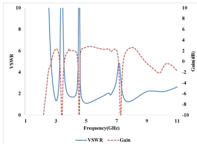
Fig. 6: VSWR and gain vs. frequency plots of the geometry shown in Figure 5.
