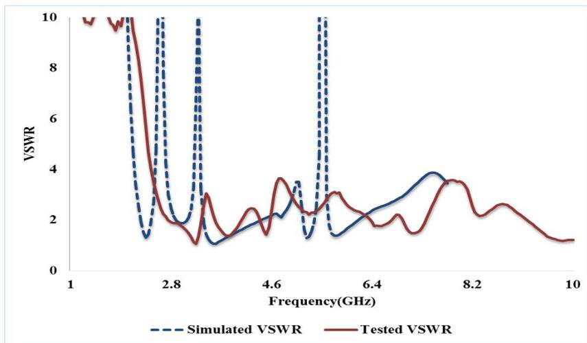
Fig. 13: VSWR vs. frequency comparisons of measured and simulated data.
