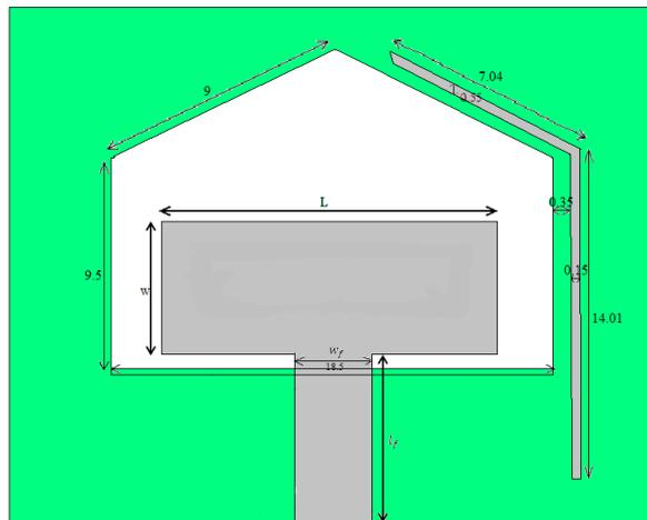
**Fig. 1:** UWB antenna geometry (all values are in mm)
