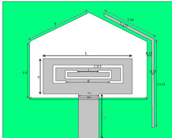
Fig. 5: UWB antenna with three notch characteristics.
