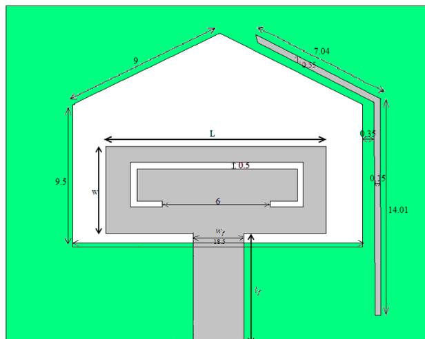
**Fig. 3:** Introduction of single notch using a metallic patch
