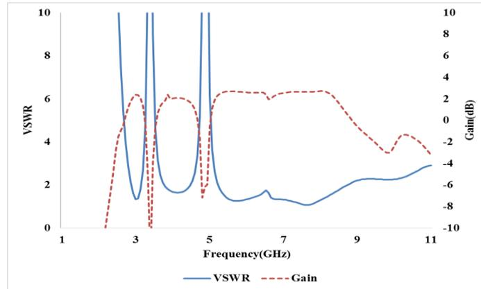
Fig. 4: VSWR, and gain vs. frequency plot of the geometry shown in Figure 3.
