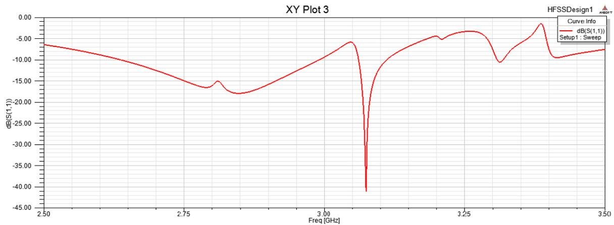
Figure 5: Return loss of proposed antenna
