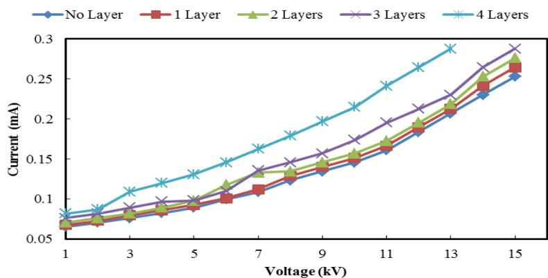
Fig. 11: Leakage current as a function of applied voltages when different layers of insulation paper are held between the electrodes in oil with 100ppm DBPC concentration.
