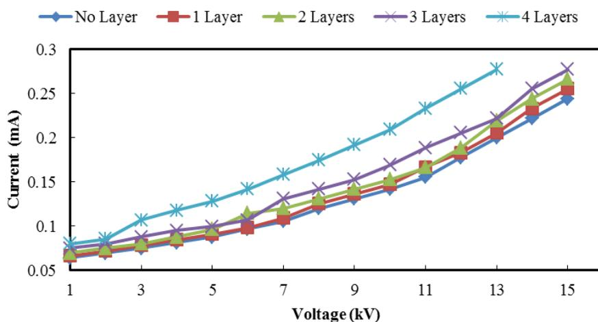
**Fig. 9: Leakage current as a function of applied voltages when different layers of insulation paper are held between the electrodes in oil with 25 ppm DBPC concentration.**
