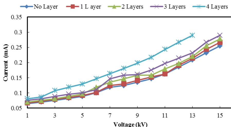
**Fig. 8: Leakage current as a function of applied voltages when different layers of insulation paper are held between the electrodes in oil with 100ppm DBDS concentration.**
