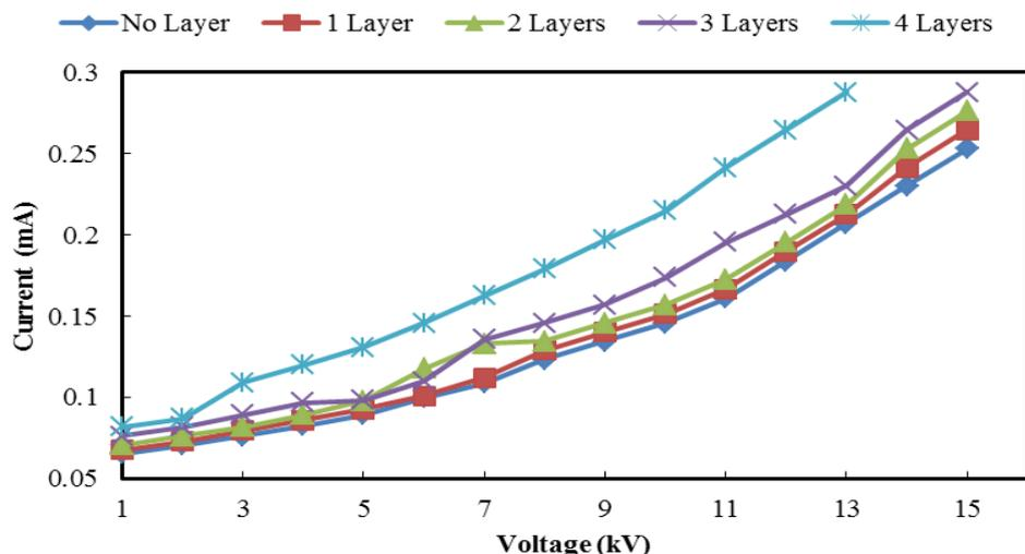
Fig. 10: Leakage current as a function of applied voltages when different layers of insulation paper are held between the electrodes in oil with 50ppm DBPC Concentration.
