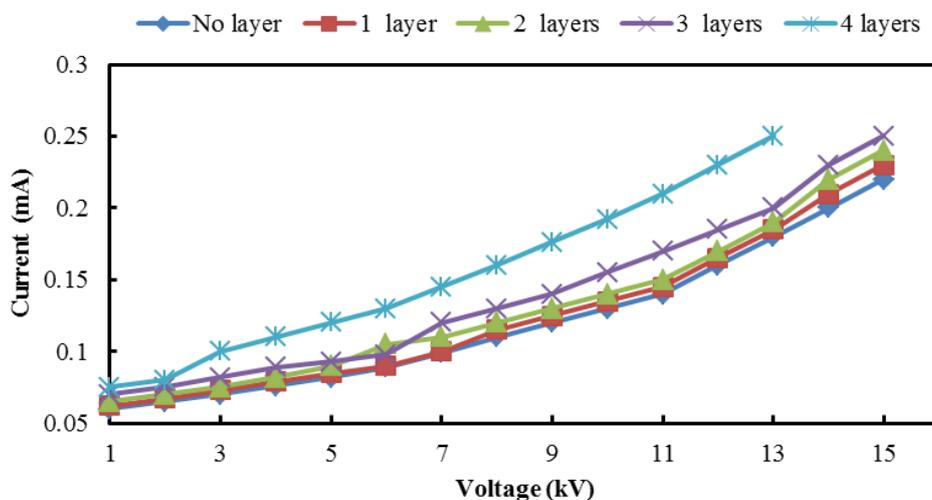
Fig. 5: leakage current versus applied voltage for clean oil having different paper layers placed between the electrodes
