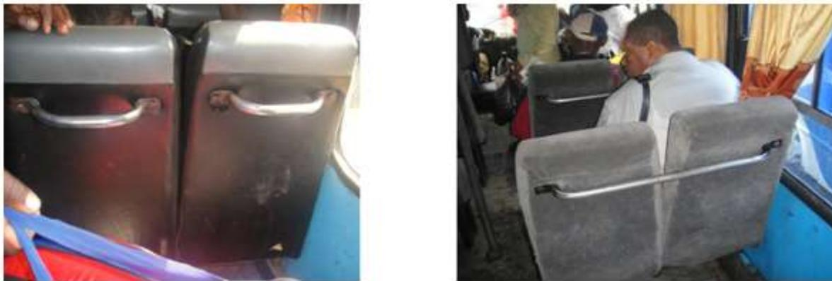
**Figure 8** Unsafe structures in bus interior may hurt passengers or cause secondary impacts
