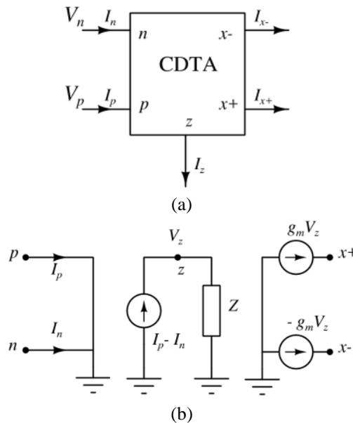
**Fig. 3** Current differential transconductance amplifier
