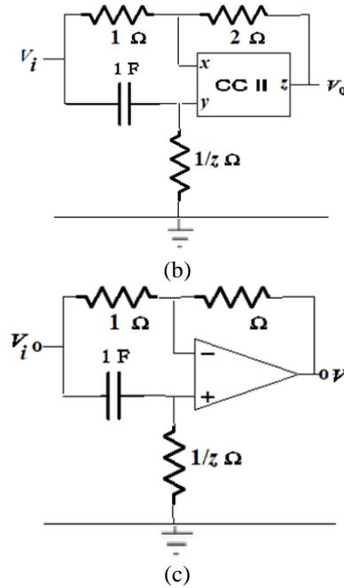
Fig. 6 Realization of voltage transfer function of (21) using (a) OTRA, (b) CCII, (c) OA
