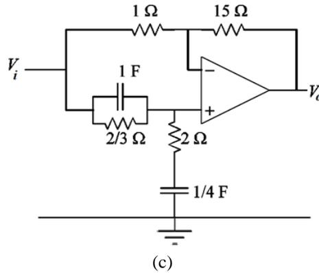
Fig. 8. Realizations of voltage transfer function of (28) using (a) OTRA, (b) CCII, (c) OA
