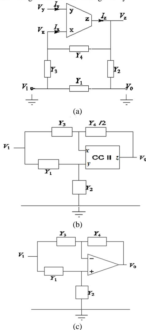
Fig. 4: Realization of voltage transfer functions using (a) OTRA, (b) CCII, (c) OA
