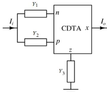
**Fig. 2:** Circuit for realizing current transfer function using CDTA
