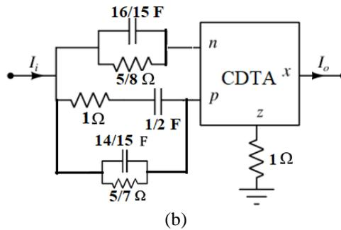
Fig. 7: Realizations of current transfer function of (28) using (a) FTFN, (b) CDTA
