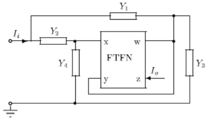
Fig. 1 Circuit for realizing current transfer function using FTFN
