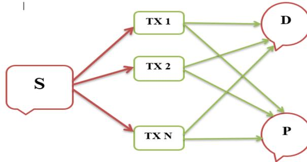
**Fig.2.1:** System model. Where all  $TX_N$  communicate with  $S$  via perfect backhaul links  $\{b_t\}_{t=1}^N$  and with both  $D$  and  $P$  via channel co-efficients  $\{h_t^d\}_{t=1}^N, \{h_t^p\}_{t=1}^N$  respectively
