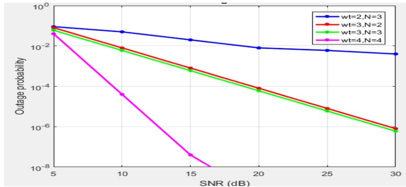
Fig 4.4: Outage probability of the proposed scheme for various values of multipath fading
