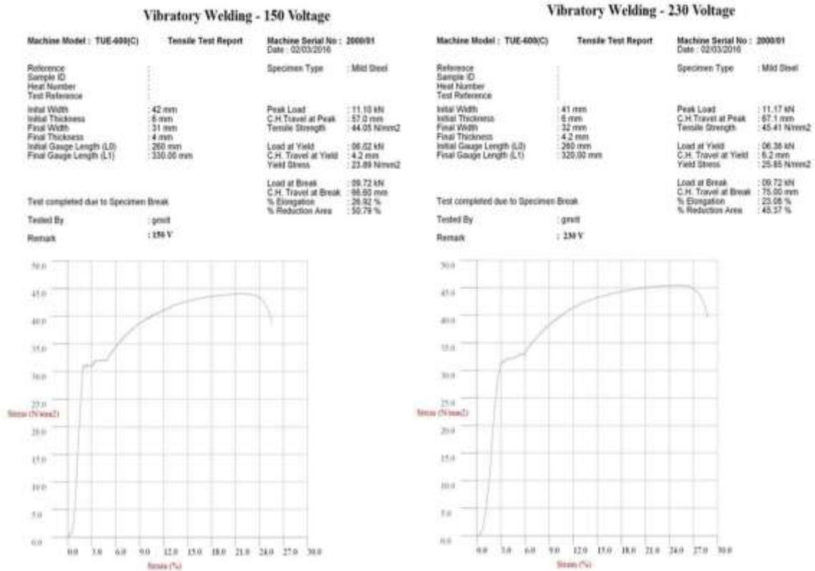
Figure 5 Sample specimen at 150v stress strain curve Figure 6 Sample specimen at 230v stress strain curve
