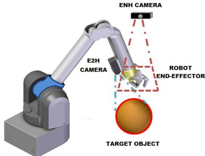
**Figure 2:** Possible Camera configurations
