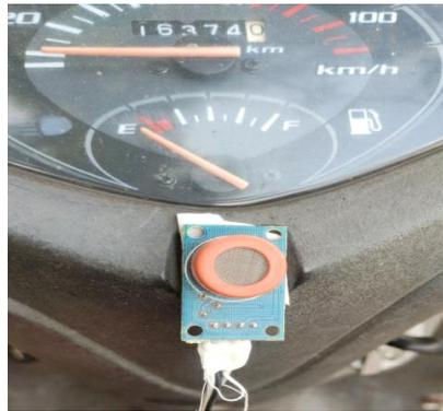
Image 3 Alcohol sensor placed on vehicle
