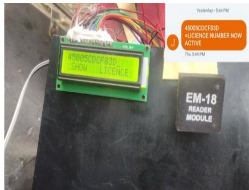
Image 7: message display on LCD as well as on which licence vehicle is running
