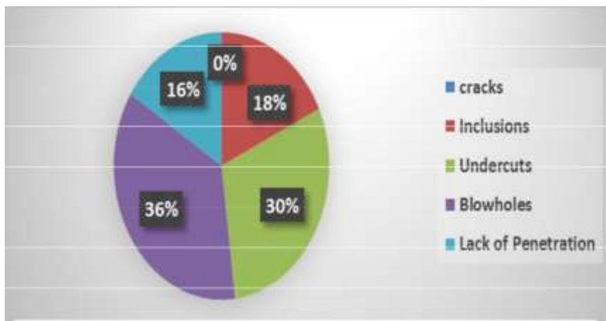
**Figure 2** Weld defects detected during NDT in different fuel tanks
