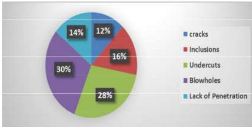
**Figure 1** Weld defects detected during NDT in different fuel tanks
