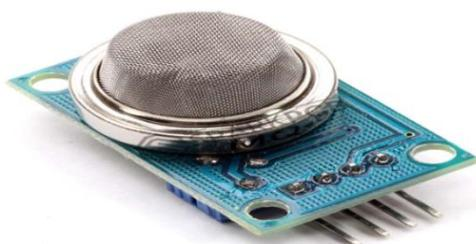
Fig.5. MQ-6 gas sensor
