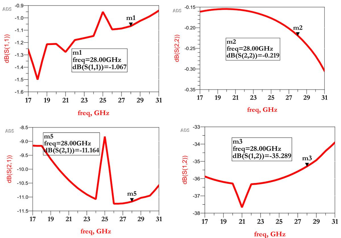
Figure 2: S parameters of the transistor
