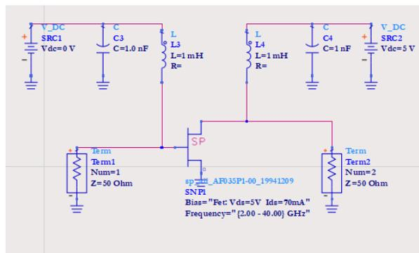
Figure 1: Schematic of the Transistor and Simulation of S parameters
