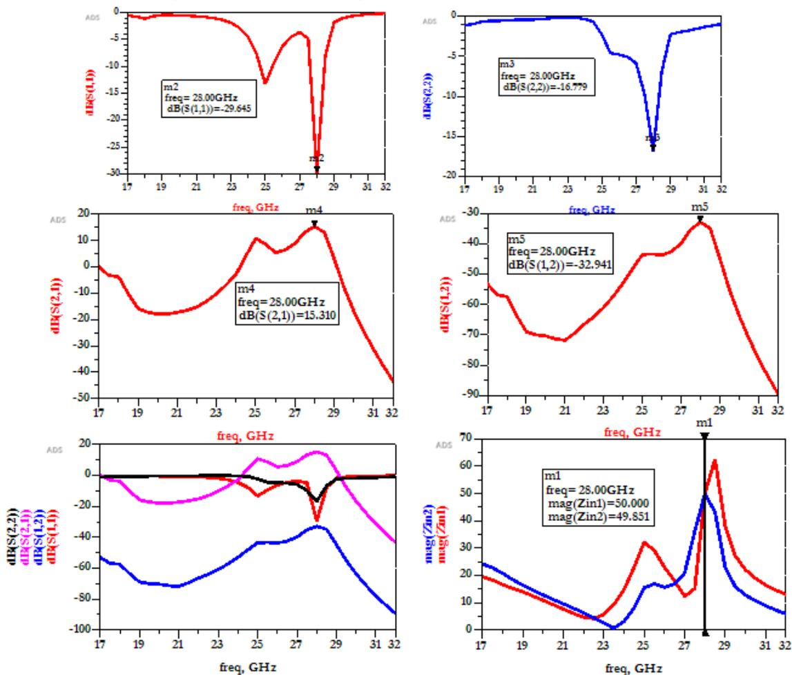
Figure 11: S Parameters and Impedance of the Amplifier with Stage
