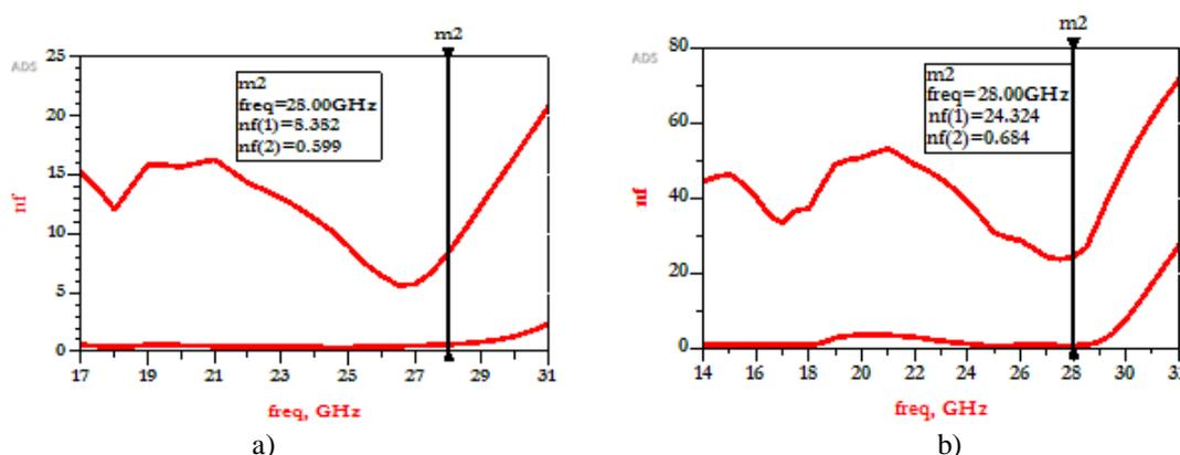
Figure 12: Microwave Amplifier Noise Factor: a) without stage, b) with stage
