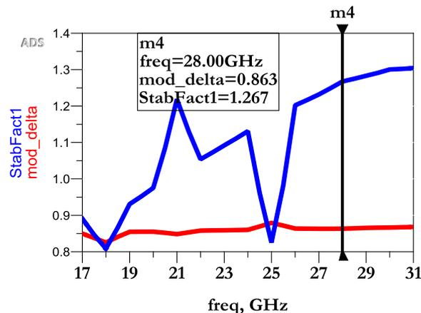
Figure 4: Parameter defining the stability of the transistor
