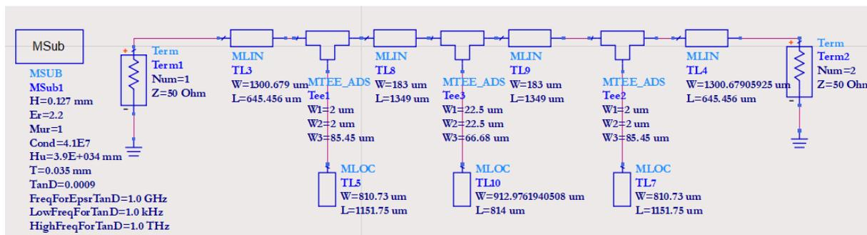
**Figure 6:** Stub structure
