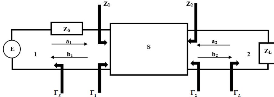
Figure 3: Distribution waves and reflection coefficients at the entry and exit of the quadrupole
