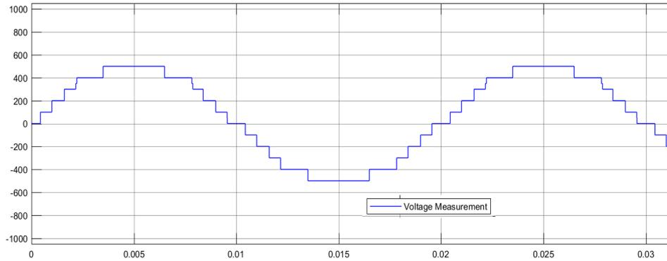
**Fig. 4:**Output voltage waveform of Two-level SHE-PWM inverter (without filter)
