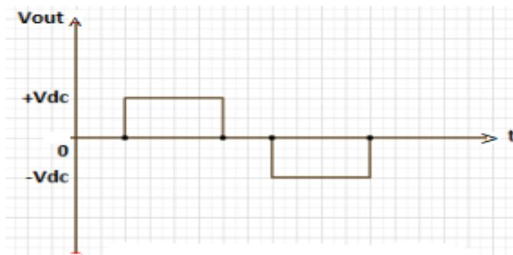
Fig.2(b). Voltage waveform of three-level inverter or a single H-bridge
