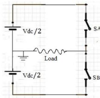
**Fig. 5(a):** A common half-bridge inverter
