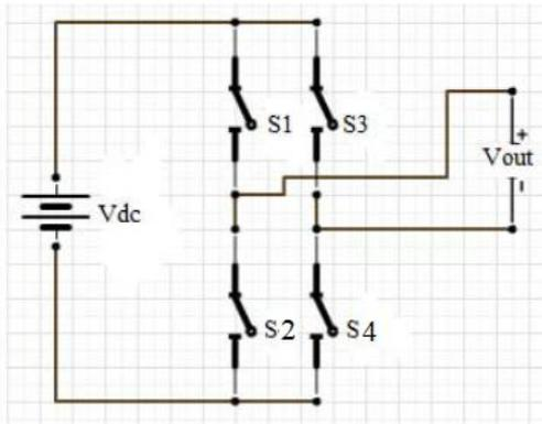
Fig.2(a). Circuit diagram of a three-level inverter
