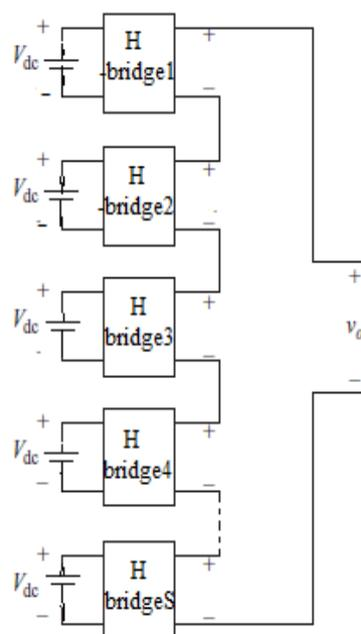
Fig.1: Multilevel Inverter with S no H-bridges.
