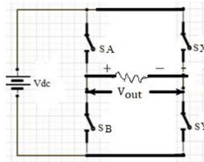
**Fig.5(b).** Circuit diagram of a three-level or H-bridge inverter
