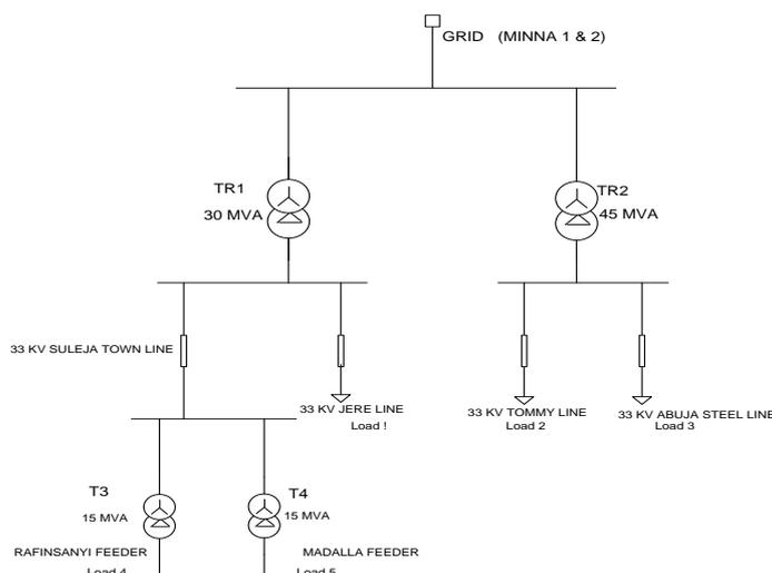
Figure 1: Single line diagram of the 132/33 kV Suleja sub-transmission power network
