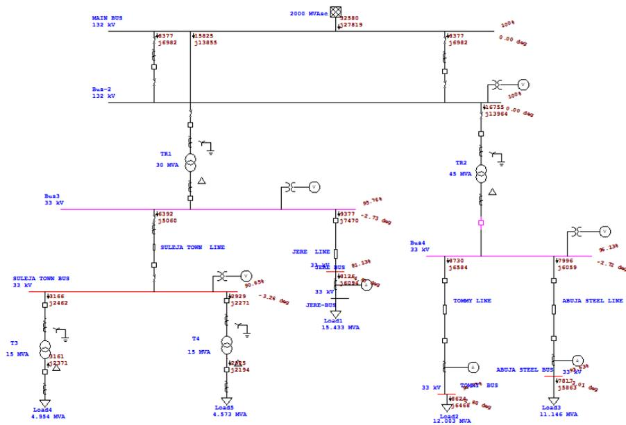
**Figure 2: Simulated model of the Suleja Substation**
