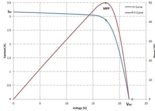
Figure 3: I-V curve and P-V curve for Bp350 PV module under STC
