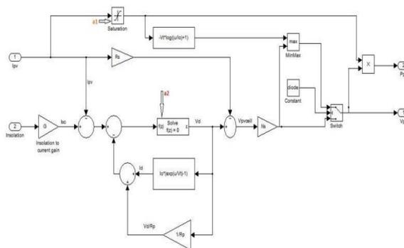
**Figure 2: Under masked subsystem of BP350 module in Simulink**
