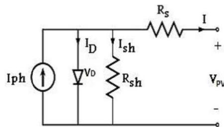
Figure 1: PV cell equivalent circuit
