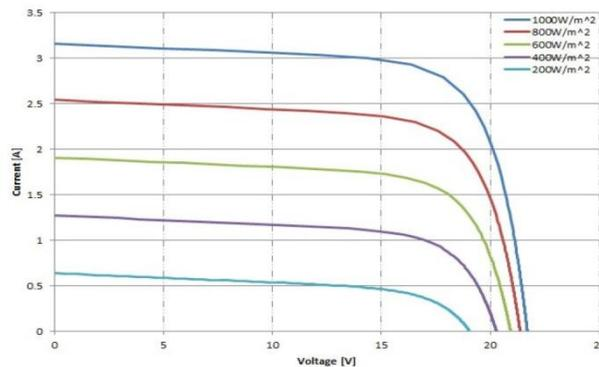
Figure 4: I-V curve for Bp350 PV at various solar insolation levels
