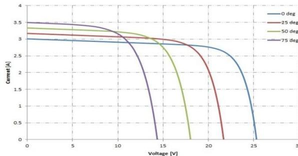
Figure 6: I-V curve for Bp350 PV at different temperature level
