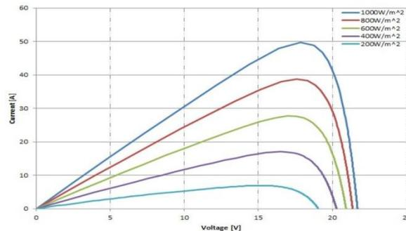
Figure 5: P-V curve for Bp350 PV at various solar insolation levels
