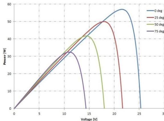
Figure 7: I-V curve for Bp350 PV at different temperature level
