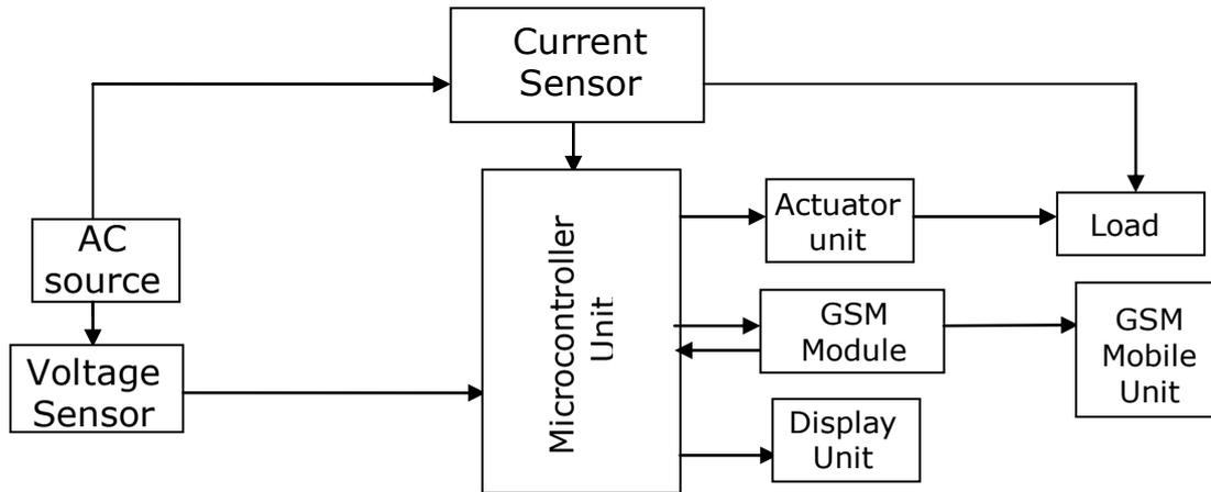
Figure 1.1: The block diagram of a smart energy meter
