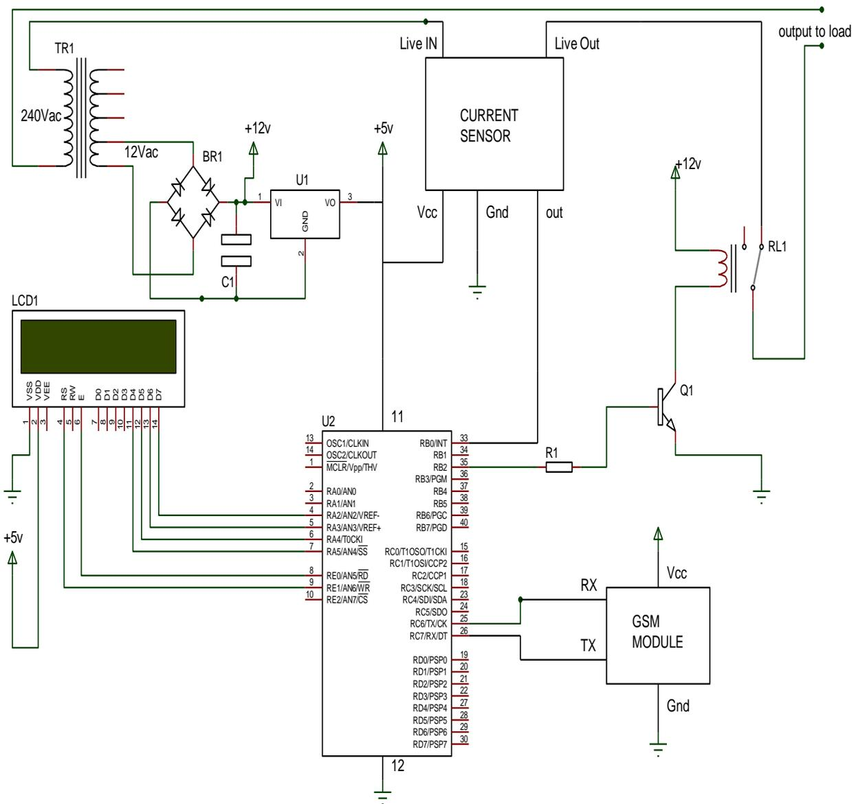
Figure 4.1: Circuit diagram of an energy meter with load control
