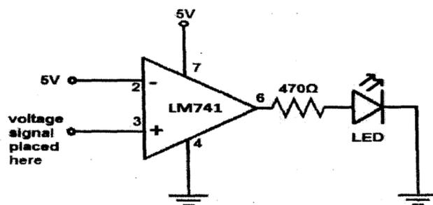
Figure 3.1: Voltage Sensor
