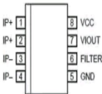
Figure 3.2: Pin-out diagram of ACS71
