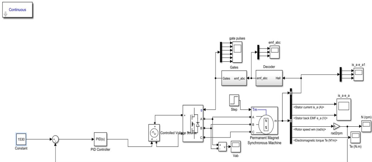
Figure no 6. Simulink Model of BLDC Motor
