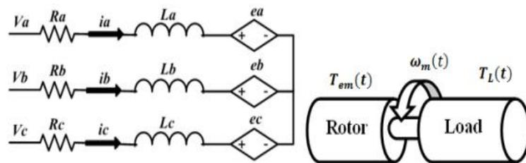
Figure no 1. BLDC motor model represents electrical and mechanical components
