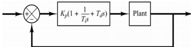
**Figure no 4.** PID Controller Block Diagram
