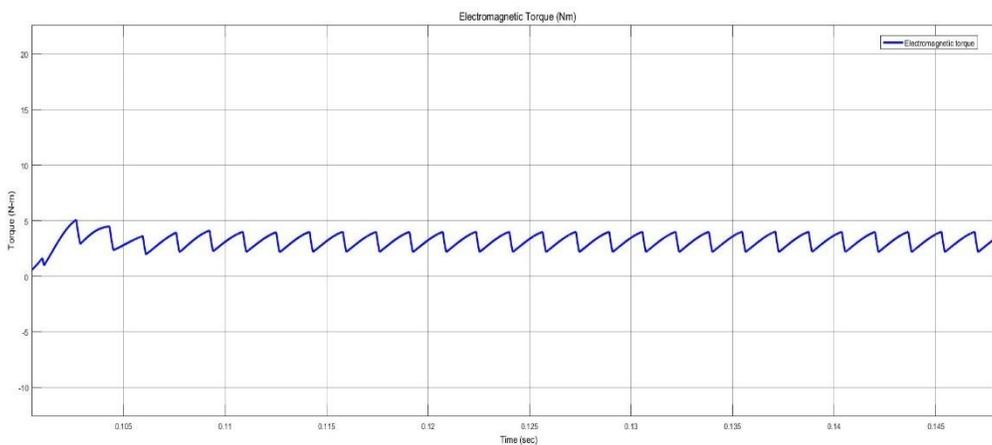
Figure no 12. Torque- Time Characteristic of the motor
