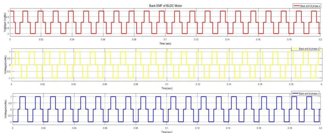
**Figure no 15.** Back EMF waveform of motor
