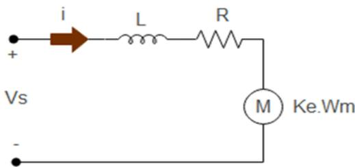
**Figure no 3** Equivalent circuit of BLDC Motor.
