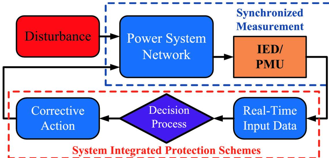
Integrated substation protection and control at the substation/plant level
