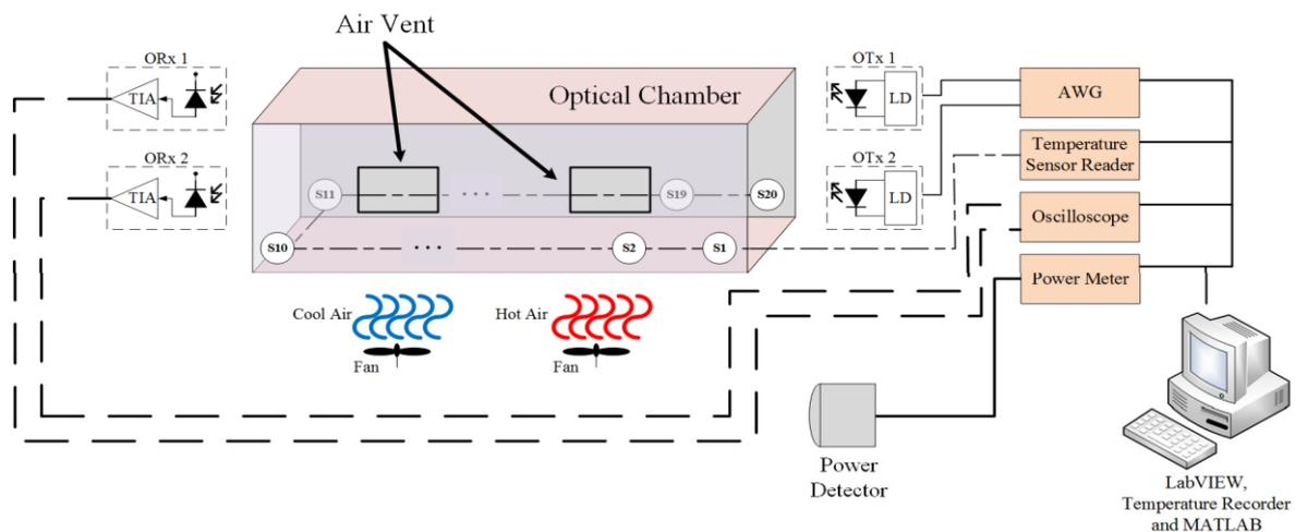
Figure 5: Diagram of the FSO arrangement.
