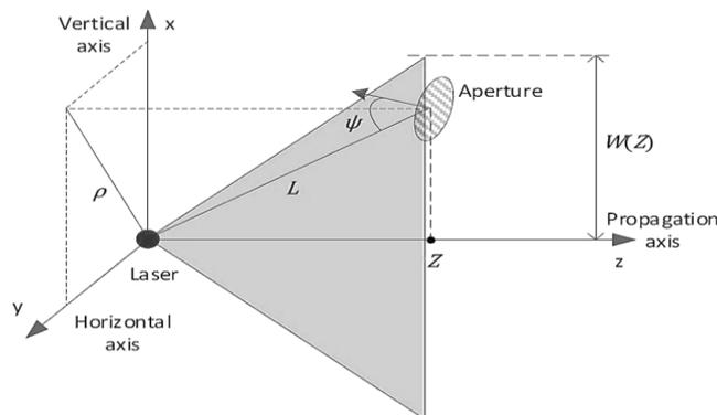
Figure 4: Laser beam and receiver aperture geometry
