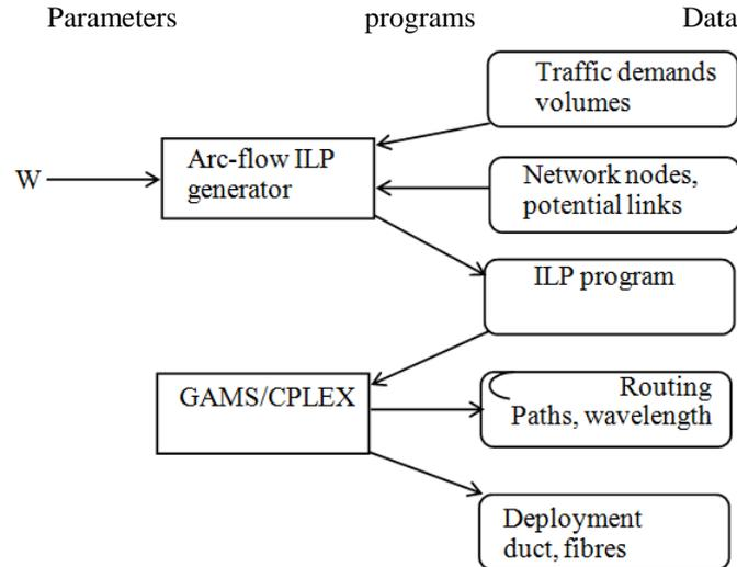
Figure 1: Optimizing WDM network using the arc-flow based ILP.
