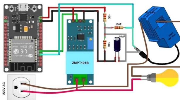
Apart from the circuit part, the AC wires where the current and voltage needs to be measured are connected to the input AC Terminal of the Voltage Sensor. Similarly, the current sensor clip doesn't have any connection and a single live wire or neutral wire is inserted inside the clip part as shown in the above circuit.
