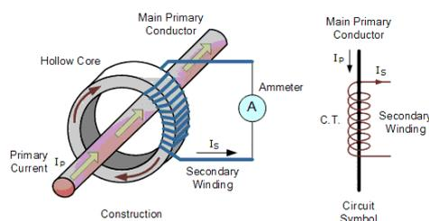
Like any other transformer, a current transformer has a primary winding, a magnetic core, and a secondary winding. The secondary winding comprises many turns of fine wire housed within the casing of the transformer.
