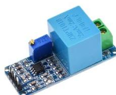
• The ZMPT101B AC Single Phase voltage sensor module is based on a high precision ZMPT101B voltage Transformer used to measure the accurate AC voltage with a voltage transformer. This is an ideal choice to measure the AC voltage using Arduino or ESP32.
