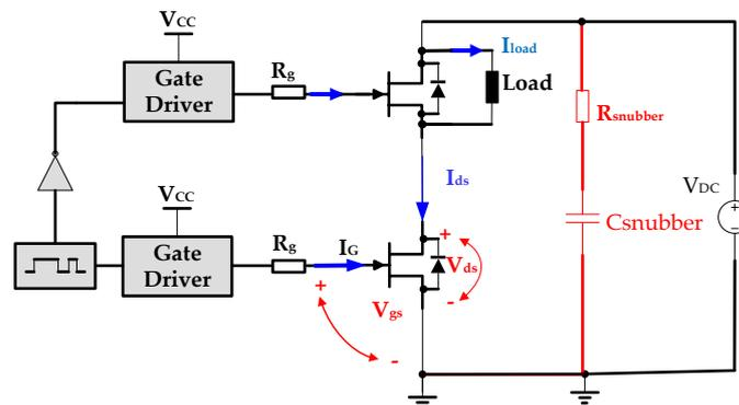
**Figure 6:** Typical DPT circuit With RC snubber.
