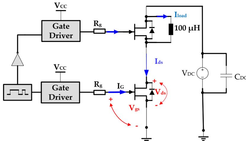
Figure 2: schematic of standard DPT.
