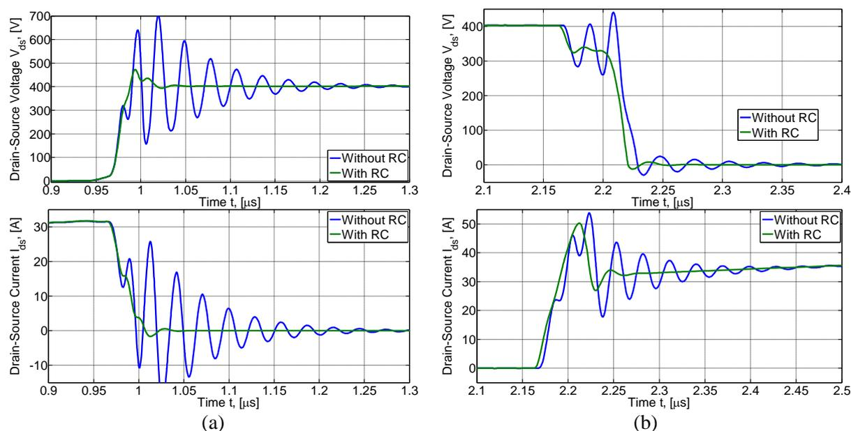
**Figure 7:** Impact of RC Snubber on Switching Oscillation: (a) Turn-on and (b) Turn-off. Test conditions:  $I_{ds}=30$  A,  $R_g=5\Omega$  and  $V_{ds}=400$  V.
