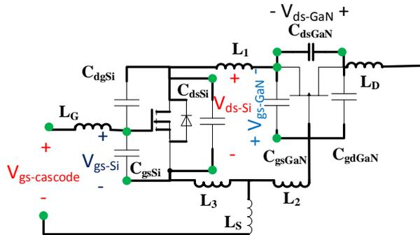
Figure 1: Schematic of cascodeGaN normally-off operation
