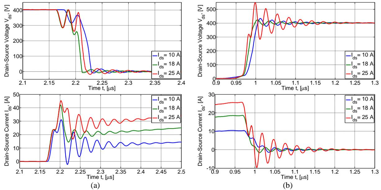
**Figure 5:** Dynamic response with different  $I_{ds}$  and  $R_g = 5\Omega$  and  $V_{ds} = 400V$ : (a) Turn-on and (b) Turn-off
