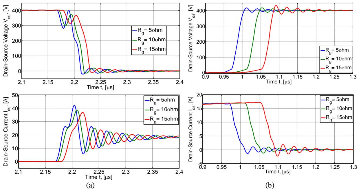
**Figure 3:** Dynamic response with different  $R_g$  and  $V_{ds} = 400$  V and  $I_{load}$  of 18 A: (a) Turn-on and (b) Turn-off
