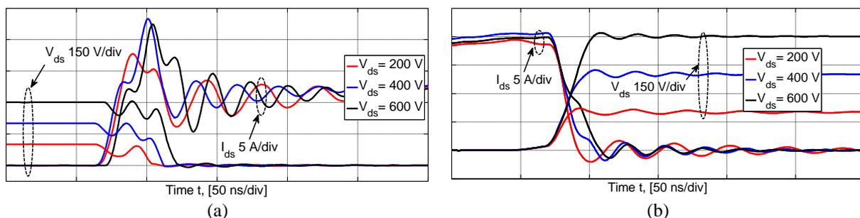
**Figure 4:** Dynamic response with different  $V_{ds}$  and  $R_g = 5\Omega$  and  $I_{load}$  of 18 A: (a) Turn-on and (b) Turn-off
