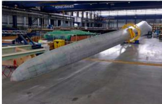
*Figure 1. V164-80m long wind turbine blade [2]*
