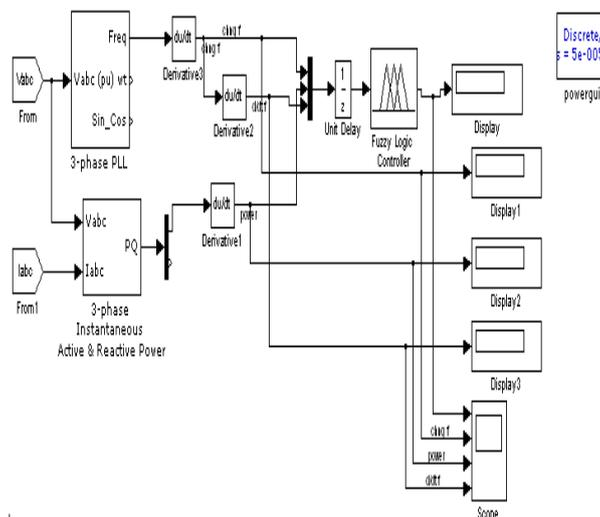
Fig.2.Fuzzy inference system for islanding detection.
