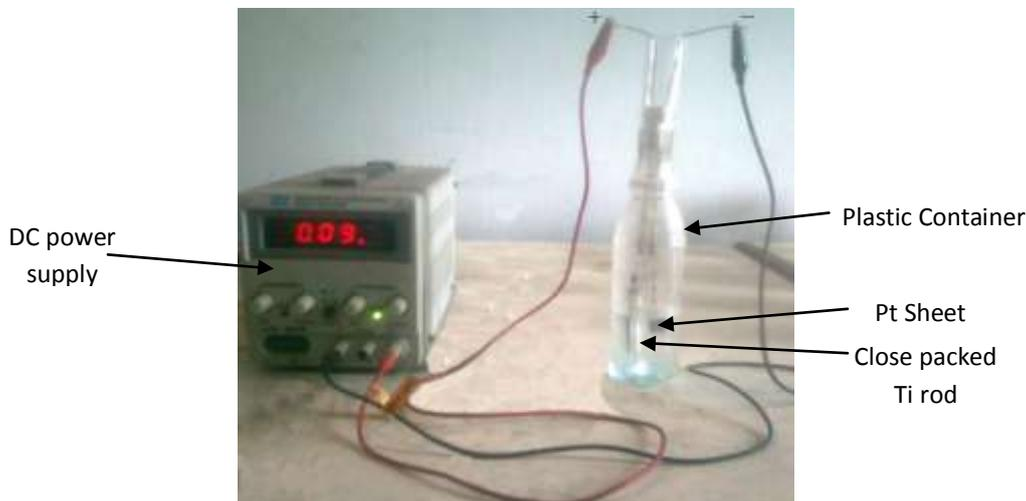
Fig. 2 An experimental setup for the synthesis of titanium dioxide (TiO<sub>2</sub>) nanoparticles by anodization
