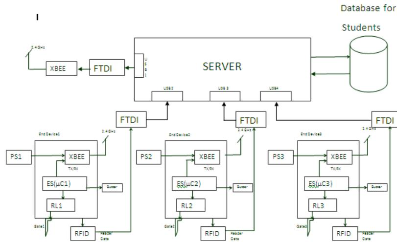
Fig1. Block diagram of Campus Security System.
