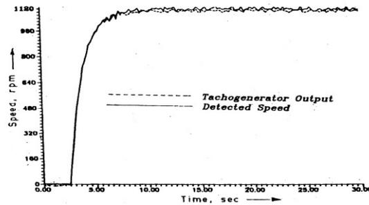
Fig. 7: Detection of Instantaneous Speed by the Imposed Method and Comparison with the Tacho generator Output (Up to Steady State)
