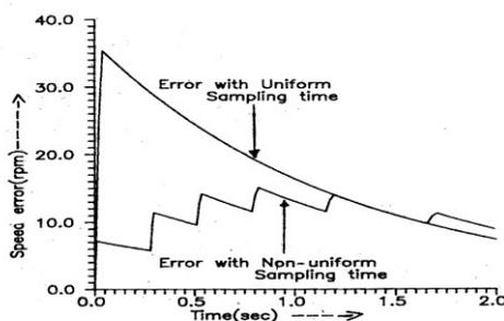
Fig. 5 (b): Comparison of Speed Error for Uniform and NonUniform Sampling Time
