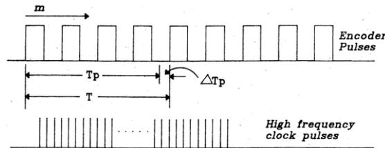
Fig. 1: Adjustment of Preset Detection Time for Integral Number of Encoder Pulses
