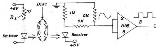
Fig. 2: Pulse Generation Circuit for the Optical Encoder
