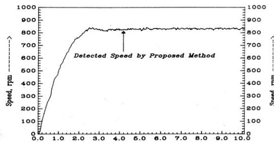
Fig. 8: the Speed rise Curve of an Inductive Motor under Vector Control Scheme using the Proposed Speed Detection Method.
