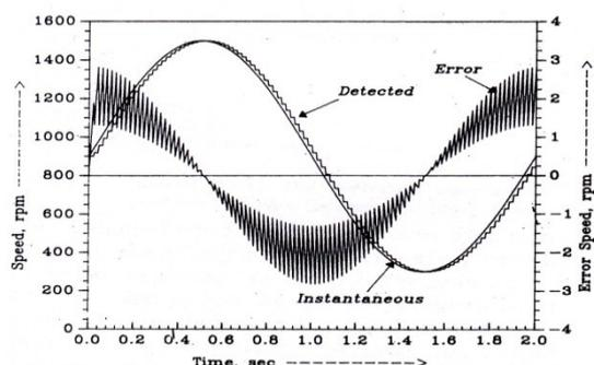
The Instantaneous all Detected Speed .Speed Error profiles for a Constant Sampling Time.
