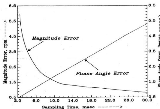
Fig. 4: Magnitude and Phase Angle Error Curves for the Proposed Method
