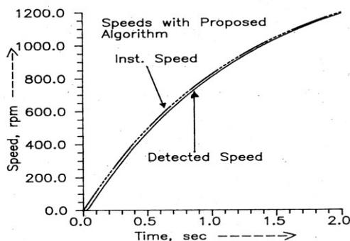
Fig. 5 (a) Instantaneous and Detected Speeds with Uniform and Non-Uniform Sampling Time
