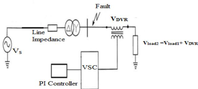
Fig.3. Overall diagram of DVR
