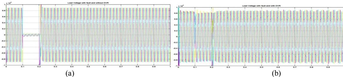
Fig.8. (a) load voltage without DVR; (b) load voltage with DVR.
