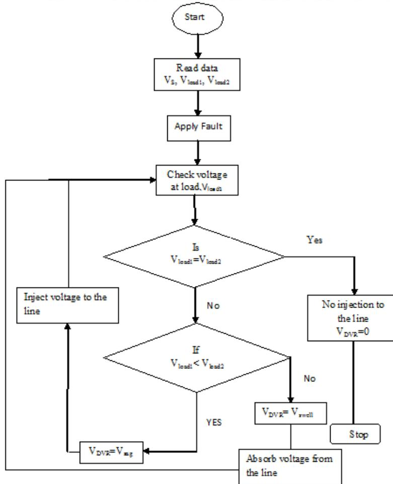
Fig.4. Flow chart of control scheme of DVR
