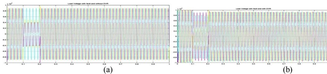
Fig.7. (a) load voltage without DVR; (b) load voltage with DVR.
