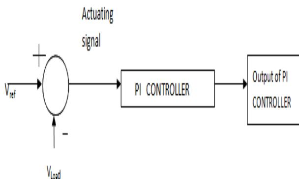
Fig.2. Operation of PI controller
