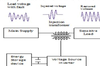
Fig.1. Operating principle of DVR
