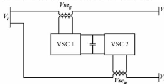
Fig: Schematic diagram of two converter IPFC
