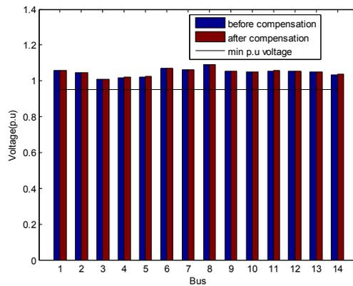
By comparing the above cases, the total power losses of the system are reduced and voltage profiles are improved by the optimal location of FACTS devices.
