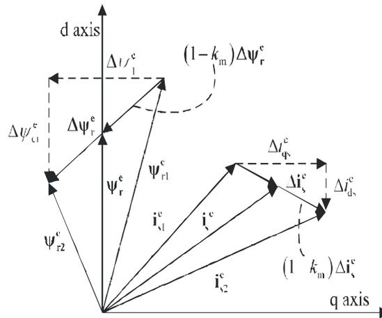
Fig 2: Weighted vector model of dual IMs fed by the single inverter.
