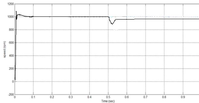
Fig.20 Speed response using PI controller in closed loop
