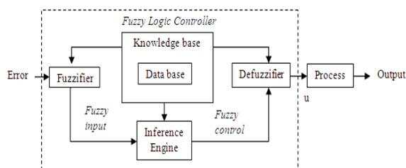
Fig. 2 Basic structure of Fuzzy Logic controller
