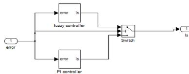
Fig.24 Simulink model of Hybrid PI- Fuzzy controller
