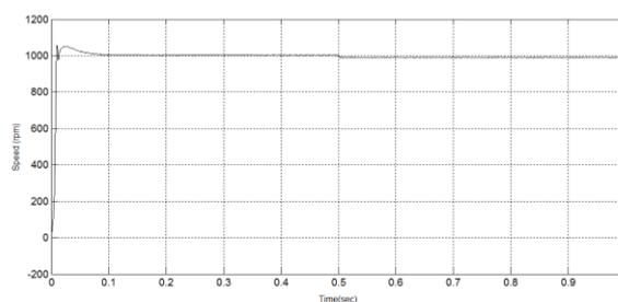
Fig.25 Speed response using hybrid PI-fuzzy controller
