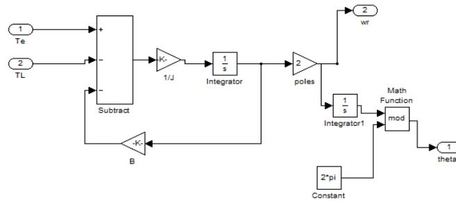
Fig.8 Simulink model for the generation of rotor speed
