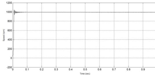
Fig.23 Speed response using fuzzy logic controller
