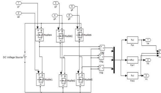
Fig.11 Voltage source inverter
