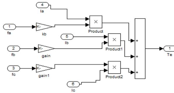
Fig.7 Generation of electromagnetic torque
