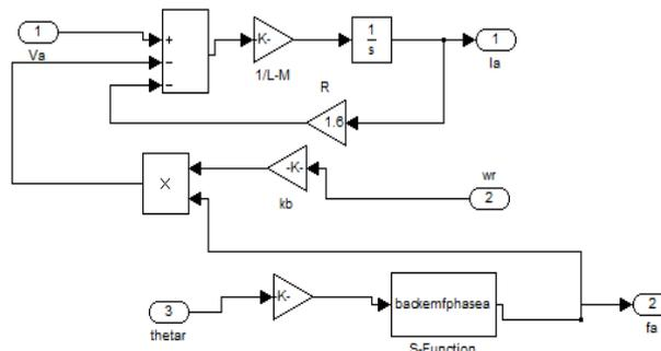
Fig. 6 Electrical block of phase a
