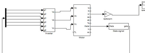
Fig.12 Simulink model of open loop BLDC motor
