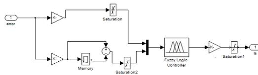
Fig.22 Simulink model of Fuzzy logic controller
