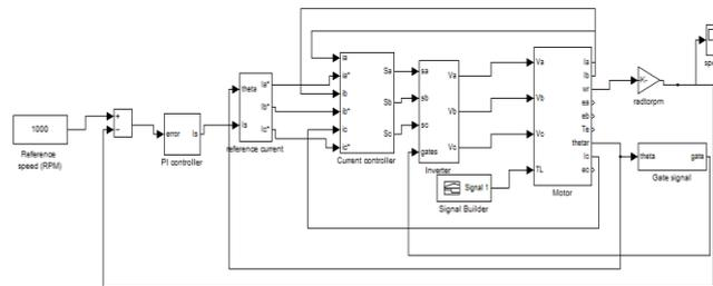
Fig.19 Simulink block of closed loop speed control using PI controller
