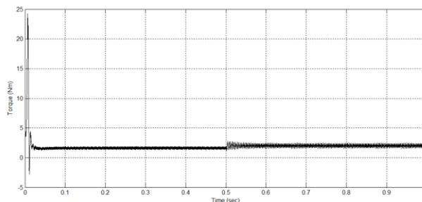
Fig.26 Electromagnetic Torque response using hybrid PI-fuzzy controller
