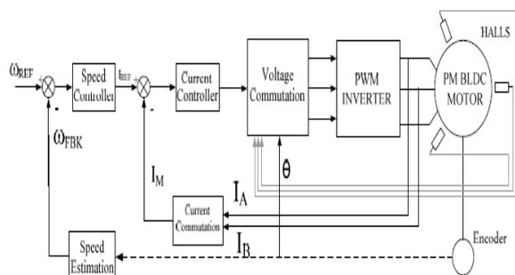
Fig. 1 Closed loop speed control of BLDC motor
