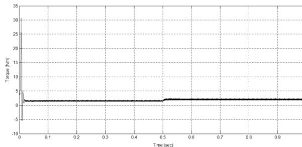
Fig.21 Electromagnetic Torque response using PI controller in closed loop
