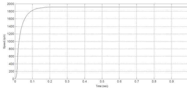
Fig.16 Open loop speed response of BLDC motor
