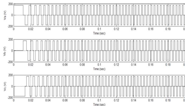
Fig.14 Voltage source inverter output
