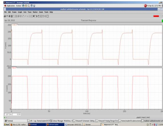
Fig 9. Design and Simulation of SUB DTMOS inverter
