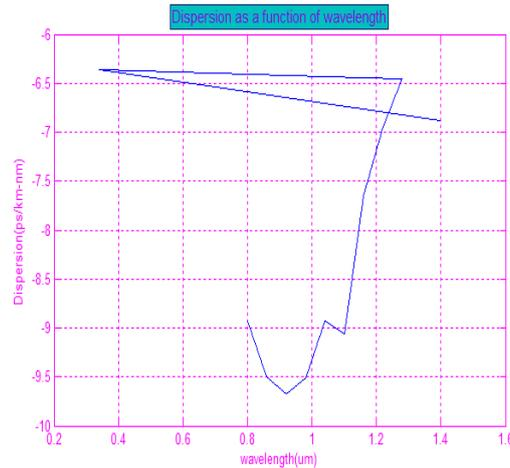
**Figure 3: Dispersion of PCF having circular shape of holes as a function of wavelength**
