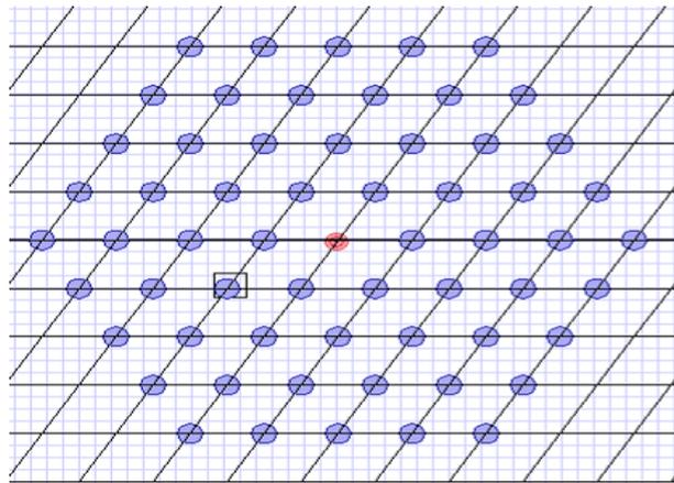
**Figure1: Hexagonal Lattice Structure of the PCF having circular shape of holes with (i) radius of 0.8 um and (ii)lattice pitch  $\Lambda=2.3\text{um}$**
