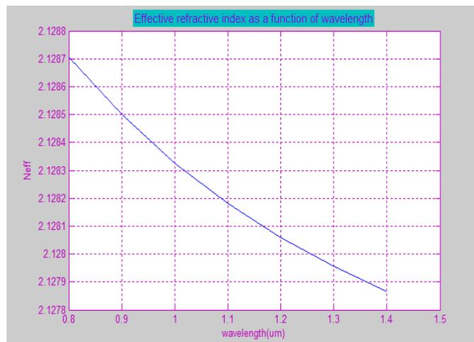
**Figure 2: Effective refractive index of a PCF having circular shape of holes as a function of wavelength**
