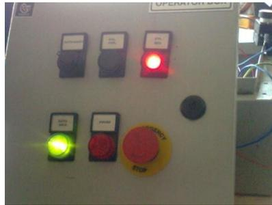
Fig.10: Operation on Pressing Cycle REV push button
