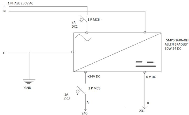
Fig. 6: Power supply Circuit
