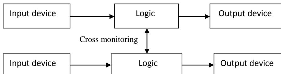
Fig. 7: Category 4 safety block diagram with cross monitoring logic
