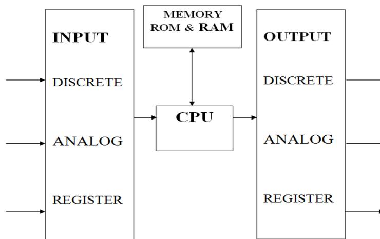
Fig. 3: Block Diagram of PLC
