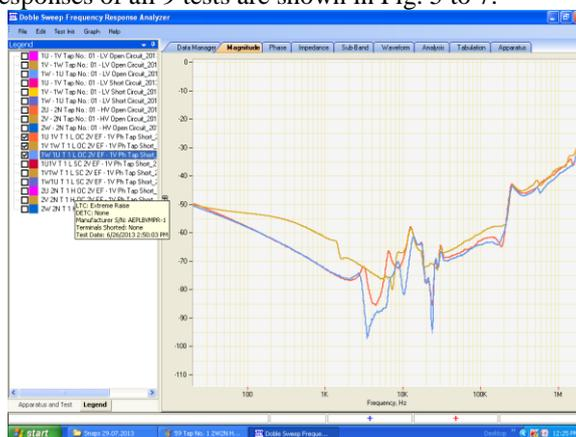
Fig. 5 Tap No. 1 HV LV Open 2V EF-1V Ph Tap Short
