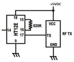
Fig. 3. RF Transmitter with Encoder
