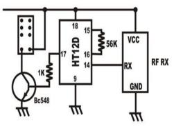
Fig. 4. RF Receiver with Decoder
