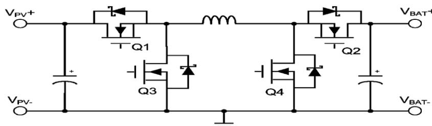
Fig. 2.2 DC/DC converter stage
