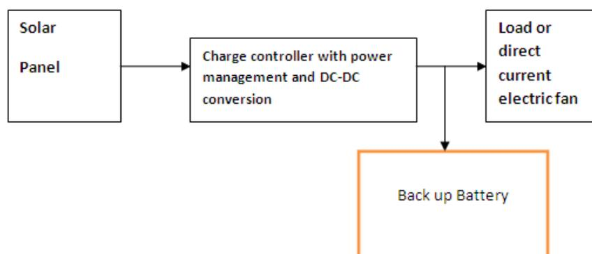
Fig. 2.3 Block Diagram of Direct Current Electric Fan Charged by Solar Panel
