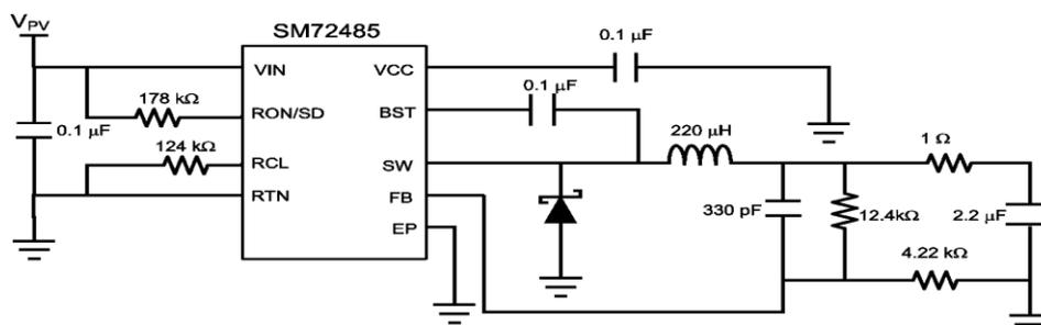
Fig. 2.1 Power Supply Circuit
