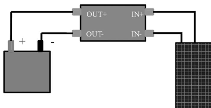
Fig. 2.0 Connection of PV and Battery to Microcontroller
