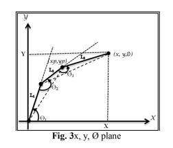
By executing the Eqn. (6), (7) & (8) using LabVIEW one can get the robot arm end-effector position. Since all the angles are measured in anti-clockwise therefore  $\theta_2 \& \theta_3$  are shows the negative angles and Eqn. (6) & (8) are modified as follows for positive angles. By executing Eqns. (7), (9) & (10) one can get the correct joint angles.
