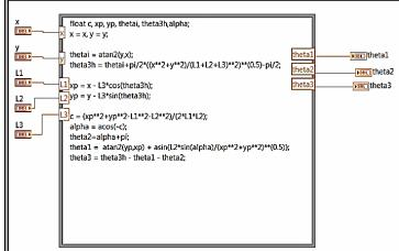
Fig. 9 Block Diagram of IK Program in LabVIEW
