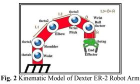
Fig. 2 shows the kinematic model of the present robot arm. Basics of trigonometry give the joint coordinates of the robot arm for position and orientation of the end effector as follows
