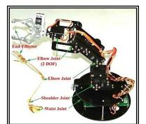
Fig. 1 Joint Configuration ofDexter ER-2 Robot Arm
