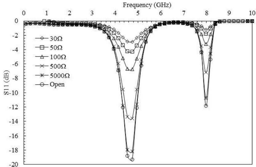
Figure:5 Variation of  $S_{11}$  when port 2 terminated with optical load and port 3 remain open
