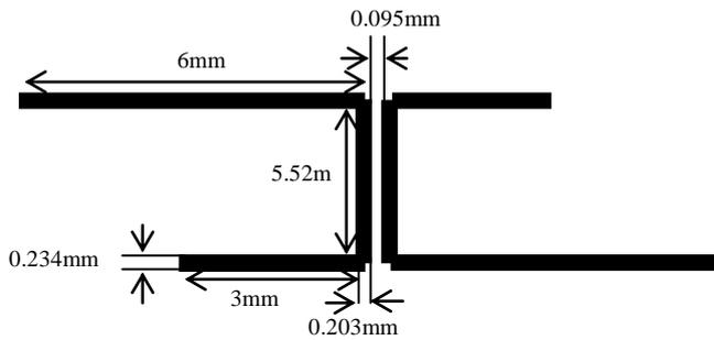
Figure:1 Optically Controlled Coupled Microstrip line Microwave Power Attenuator
