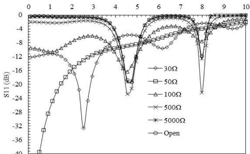
Figure:9 Variation of S11 when both port 2 and port 3 terminated with optical load
