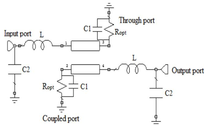
**Figure:2** Equivalent Circuit of Optically Controlled Coupled Microstrip line Microwave Power Attenuator with the SMA to microstrip transition.
