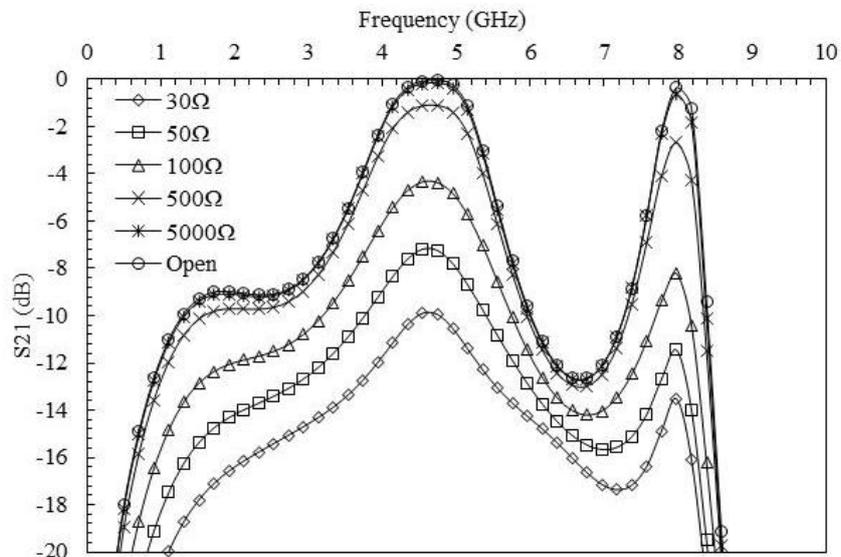
Figure:6 Variation of  $S_{21}$  when port 3 terminated with optical load and port 2 remain open
