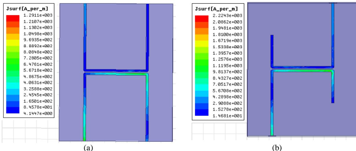
**Figure:3** Current density distribution in (a) primary directional coupler and in (b) optically controlled attenuator when both port open (maximum power at port four)
