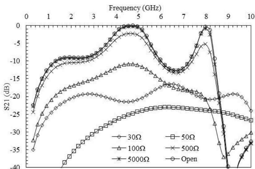
Figure:8 Variation of S21 when both port 2 and port 3 terminated with optical load
