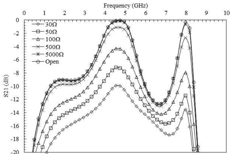
**Figure:4** Variation of S21 when port 2 terminated with optical load and port 3 remain open
