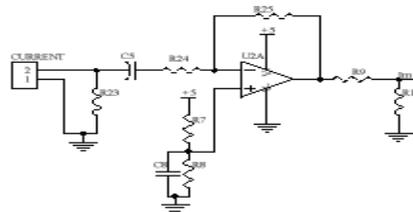
**Figure 4:** Circuit Diagram for Current Detection
