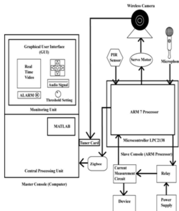
**Fig 2:** Block Diagram
