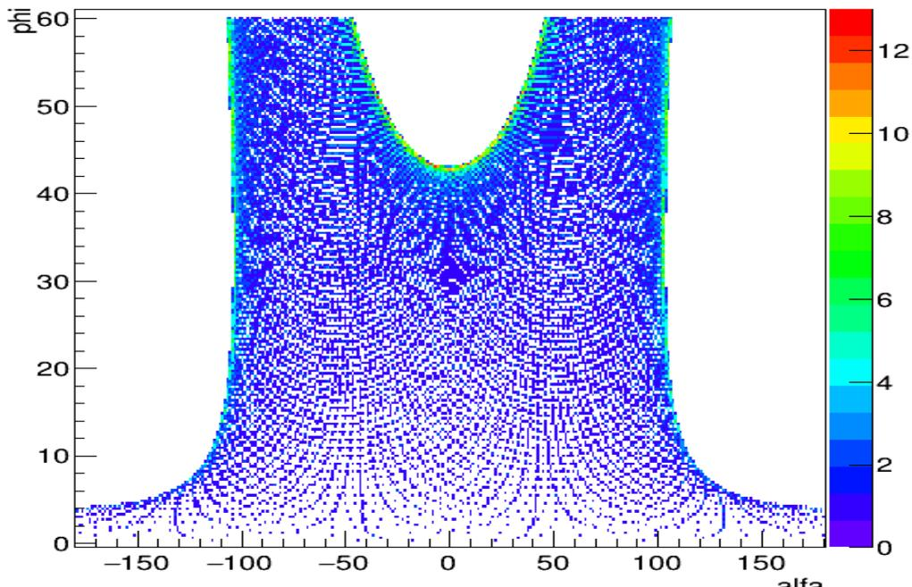
Fig 4: Sun position in zenith angle ( $\phi$ ) and azimuthal angle (“alfa”) to Mexico City
