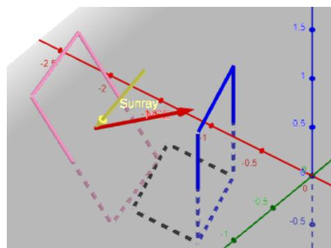
**Fig 3:** Representation of the solar ray (Sunray yellow), normal to the mirror (NSE red)
