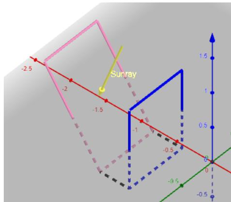
**Fig. 2:** Lens (blue) and mirror (pink) placement according to the melting point (point at (0,0,0)) and the solar position (yellow)
