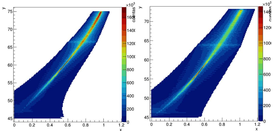
Fig 8: Left: mirror at  $0^\circ$  from negative x axis, right: mirror at  $56^\circ$  from negative x-axis. Distance (x in m) vs rotation angle (y in  $^\circ$ ) of both cases.
